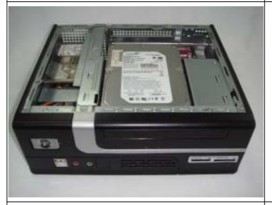
(3) Before installing back the Front Panel onto the Chassis, - Secure the Slim ODD's Plastic Bay Cover,
