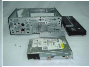
(1) Before assembling the systems, Dismantle the Front Panel from the Chassis Frame,
