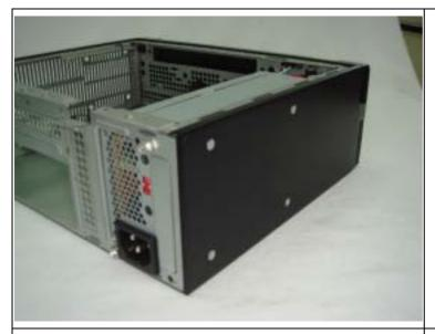
(5) Use 4 pcs of M3\*0.5p\*L5 Flat Head Screw to secure the 2.5" HDD from the external side of Chassis.
