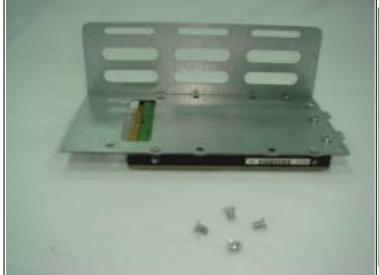
(3) Use 4 pcs of M3\*0.5p\*L5 Flat Head Screw to -Secure the 2.5" HDD on top of the Upper Fixture Bracket.
