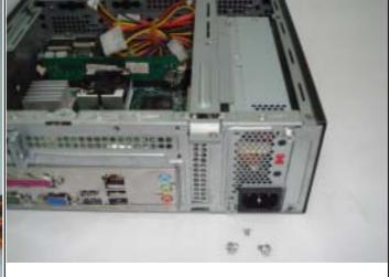
(1) The Fixture Bracket is not required for the installation of the (2) Position the Power Supply in the case, - FSP150-50AF Model Power Supply.
