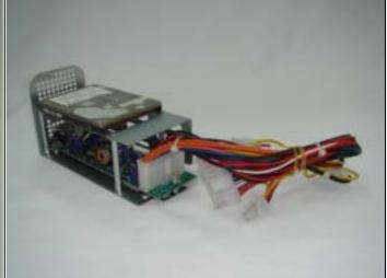
(4) Use 4 pcs of 6-32\*L4 Flat Head Screws to -Secure the assembled Upper Fixture Bracket on top of the 4 Long Pillar Posts of the Lower Fixture Bracket.
